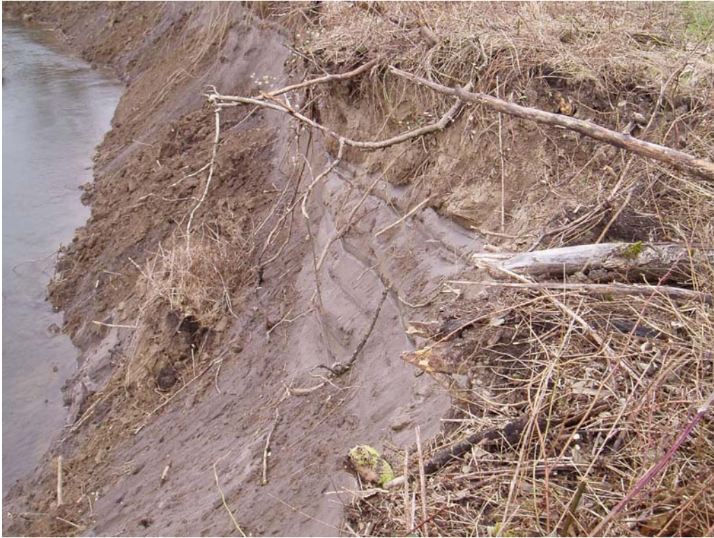
Figure 6.5. Silty loam layer on bank of the Sandy River Delta.
