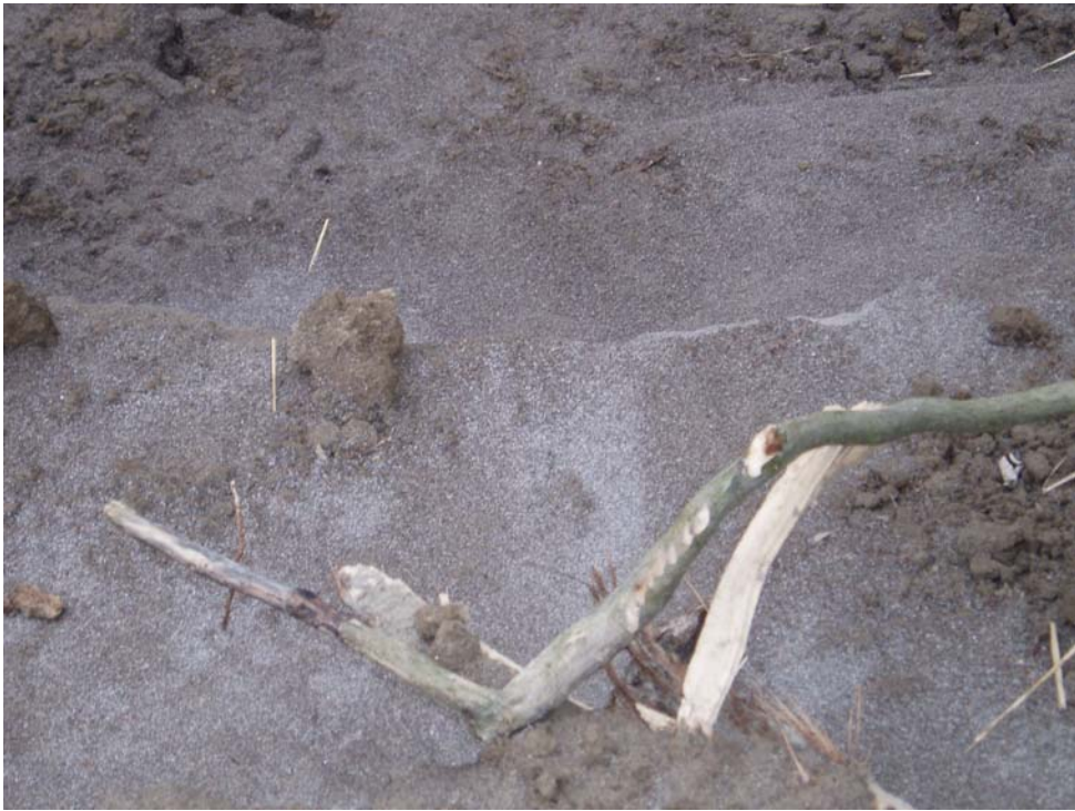
Figure 6.7. Non-cohesive loam that comprises the bank.
