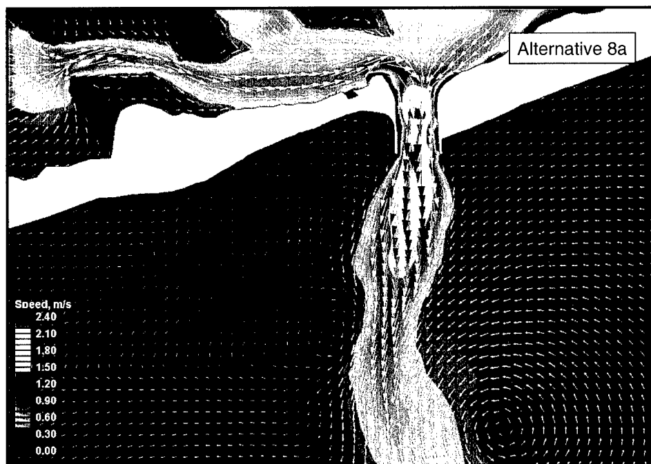
Figure 61. Alternative 8a velocity vectors and speed at inlet and ebb shoal, peak ebb tide
