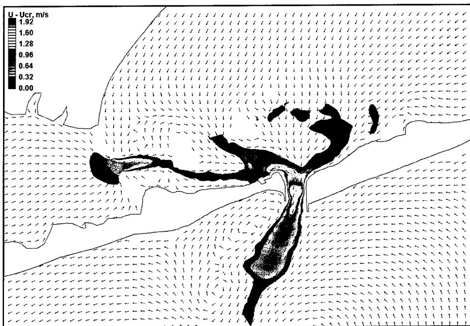
Figure 70. Excess suspension speed at peak ebb tide for Alternative 5
