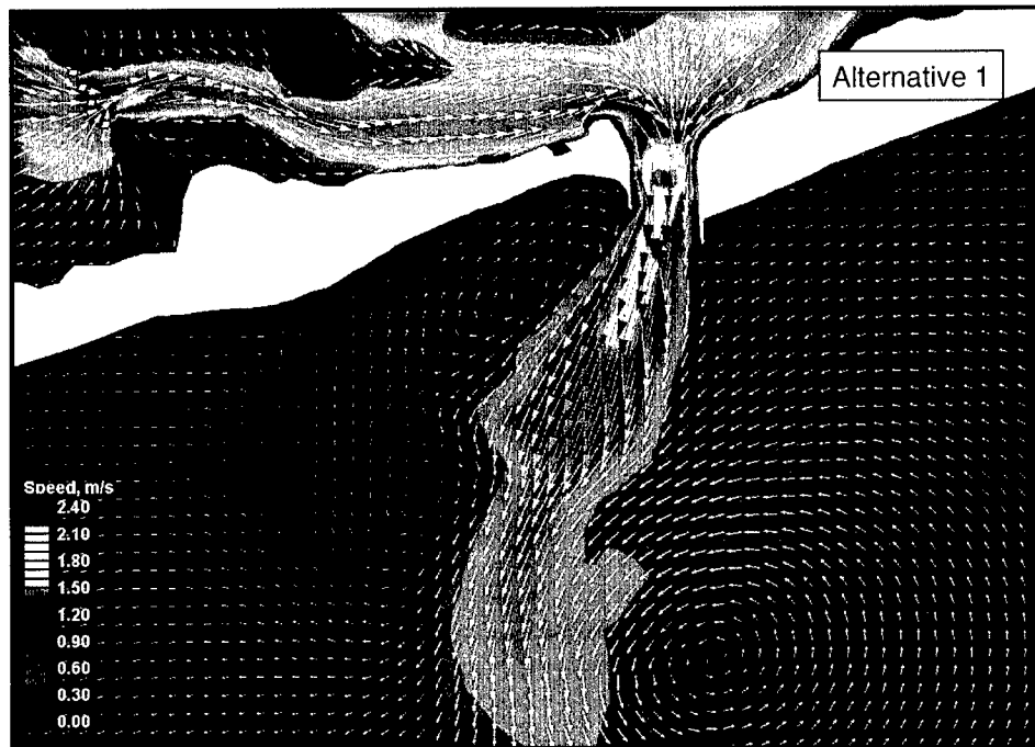
Figure A6. Alternative 1 velocity vectors and speed at inlet and ebb shoal, peak ebb tide
