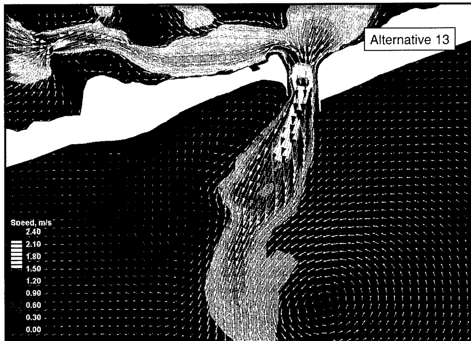
Figure A48. Alternative 13 velocity vectors and speed at inlet and ebb shoal, peak ebb tide
