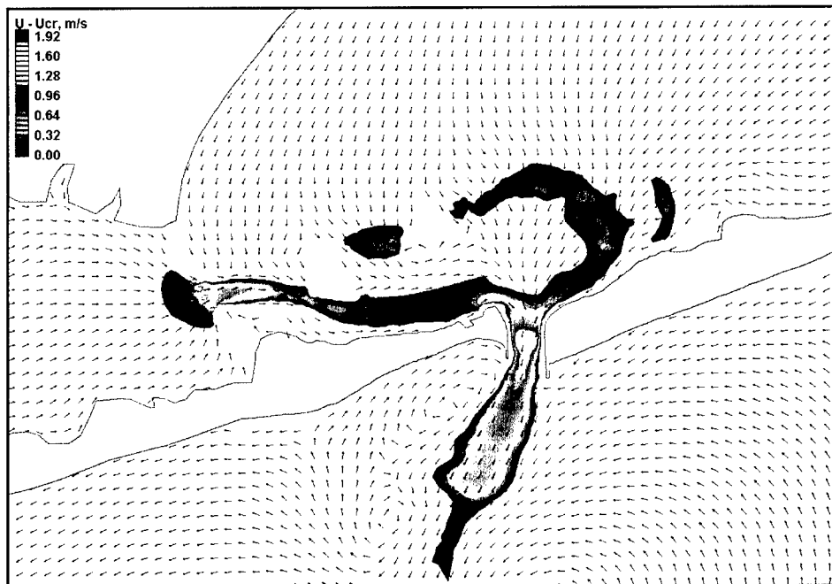
Figure 68. Excess suspension speed at peak ebb tide for Alternative 1
