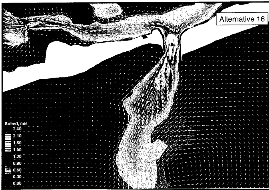
Figure C8. Alternative 16 velocity vectors and speed at inlet and ebb shoal, peak ebb tide
