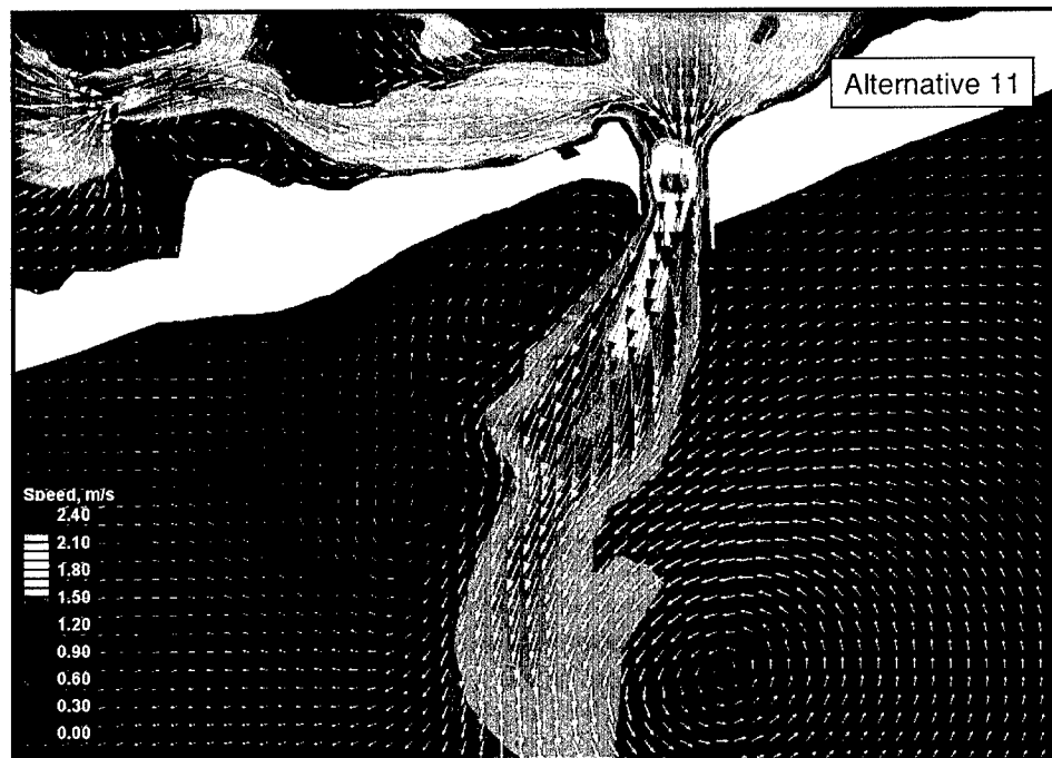
Figure A42. Alternative 11 velocity vectors and speed at inlet and ebb shoal, peak ebb tide
